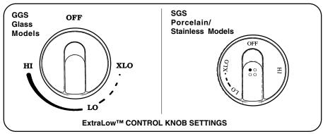
Both ExtraLow controls are push in to turn and have an infinite number of heat settings, with no fixed positions. The ExtraLow settings are between **XLO** and just after **LO**, at the detent, shown by the broken line.
